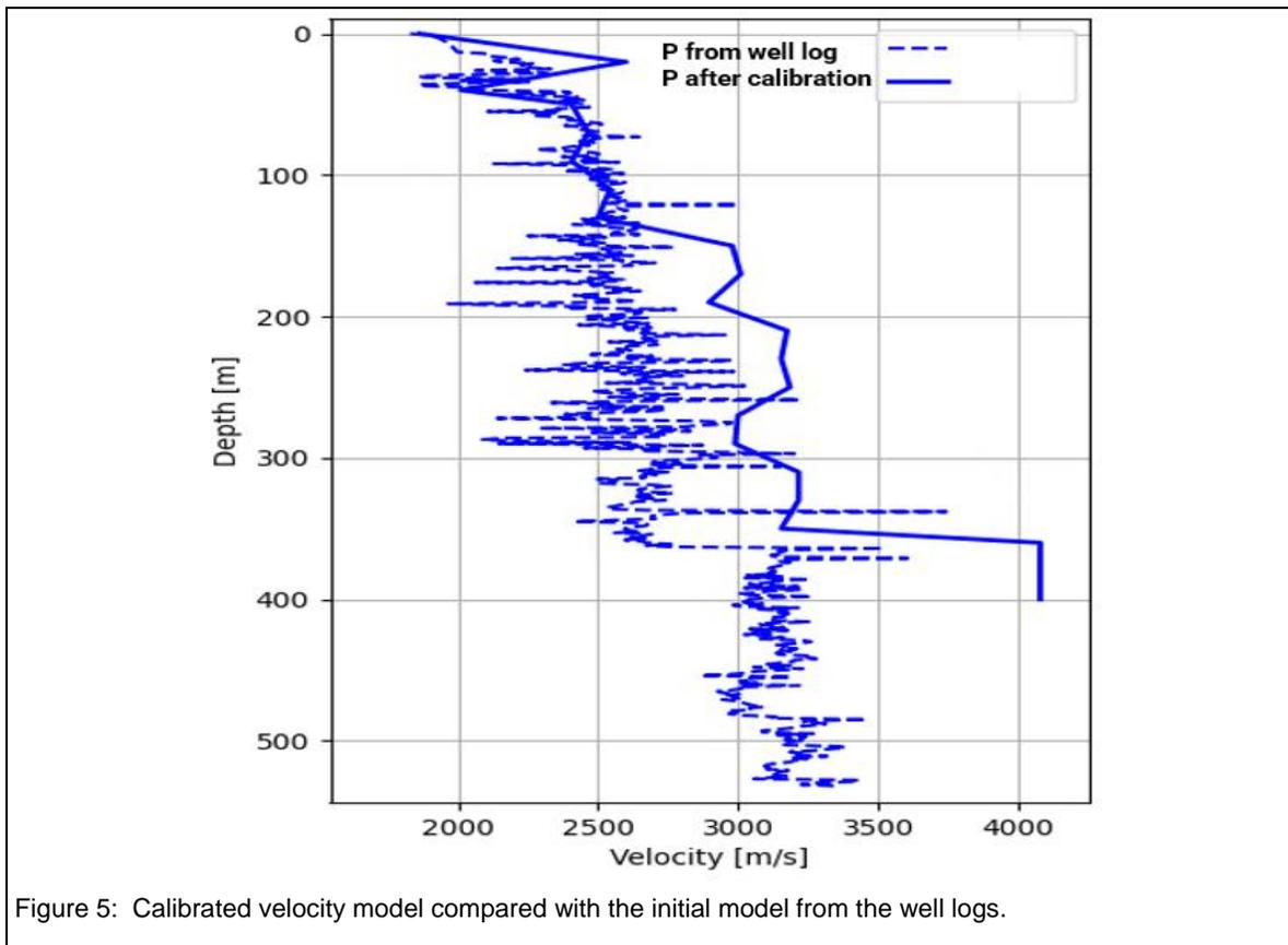
Figure 5: Calibrated velocity model compared with the initial model from the well logs.
