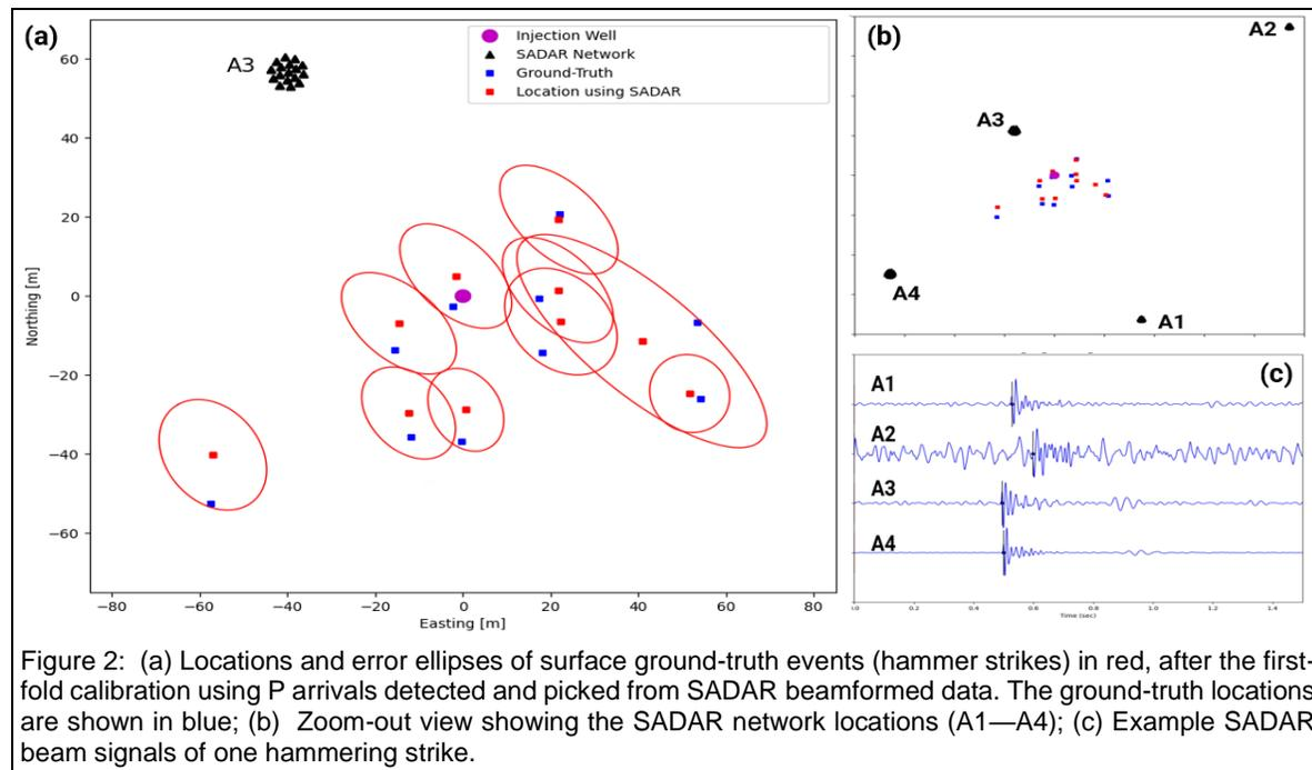
Figure 2: (a) Locations and error ellipses of surface ground-truth events (hammer strikes) in red, after the first-fold calibration using P arrivals detected and picked from SADAR beamformed data. The ground-truth locations are shown in blue; (b) Zoom-out view showing the SADAR network locations (A1—A4); (c) Example SADAR beam signals of one hammering strike.
