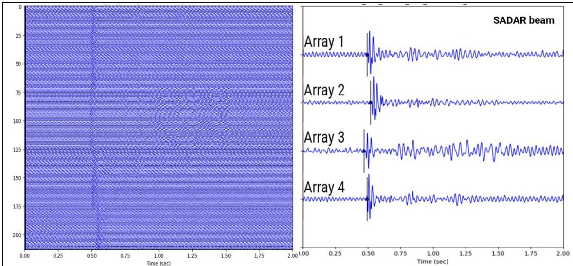
Figure 4: (left) Signals across all individual channels of the SADAR arrays; (right) optimal beam signals for network of four SADAR arrays.
