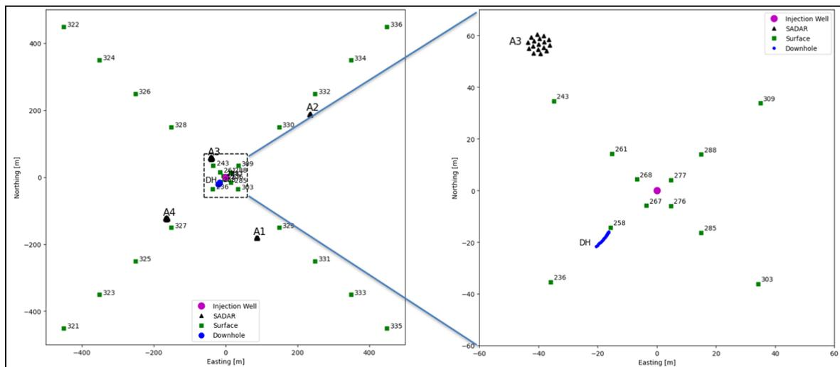
Figure 1: (left) Map view of the seismic monitoring networks centered at the injection well (magenta dot at center), and showing the locations of the SADAR arrays (A1—A4, black triangles), the surface network (green squares), and the downhole array (blue dots). (right) Zoomed-in map view of the area close to the injection well.
