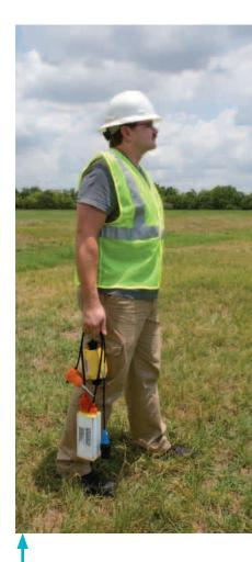
Small, light and minimally invasive cableless technologies like the OYO Geospace GSR system are transforming how seismic data is acquired.
