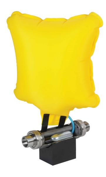
The Universal Inline SRD is an automatic, sealed Streamer Recovery Device that aids in the recovery of seismic marine streamers which have been accidentally severed from a tow vessel. These devices are placed at specified intervals (300 meters maximum) inline with the streamer cable and are activated when the streamer sinks to a preset depth of approximately 48–60 meters or pressure of 70–87.5 psi.
