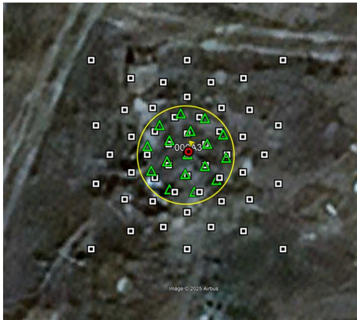
Figure 4. (left) Spatial view of the Array 3. The SADAR borehole sensors are located at the positions of the triangles (green), buried at depths of 9, 11, and 13 m. The surface patch array are shown at the positions of the squares (white). (right) Spectra calculated for the surface sensors and buried SADAR sensors. The top shows individual sensor; the bottom shows the results of the beam.
