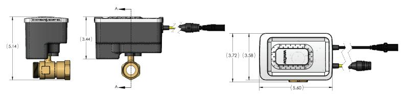
Meter cable shown above is an option for the AquaFlow valve when reading a meter is desired.
