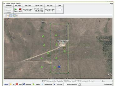
Surface sensor systems (green triangles) detecting and locating miners (blue "X") over 1000' underground inside a very large, active, long seam coal mine.
