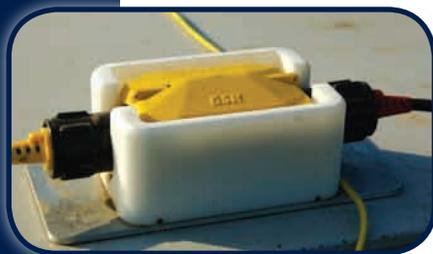
*OYO Geospace provides shot controllers for any field energy source used. Synchronized to a GPS clock, they provide the most accurate shot timing available.*
