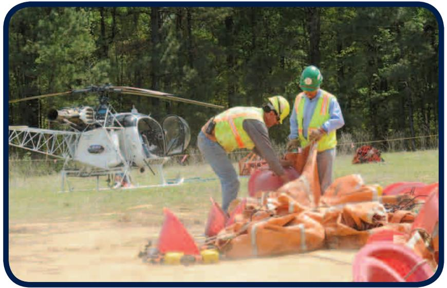
To image this area, Dawson is using vibrators, airguns and dynamite sources – whichever is appropriate to the varying conditions in the field. For receivers, they’ve used the Aram system in the transition zone and now are completing the land portion of the survey using OYO’s Geospace Seismic Recorders (GSRs).
