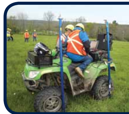
The ATV-mounted mobile control console can also be hand carried and avoids large “doghouses” needed for cabled systems.
