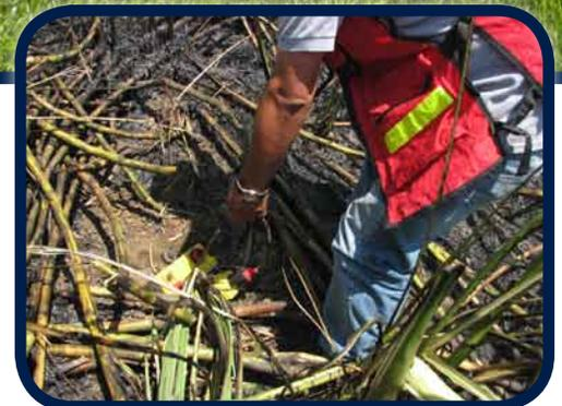
*Burial allowed the GSR units to avoid field fire damage – even buried the GSRs continued to operate perfectly.*
